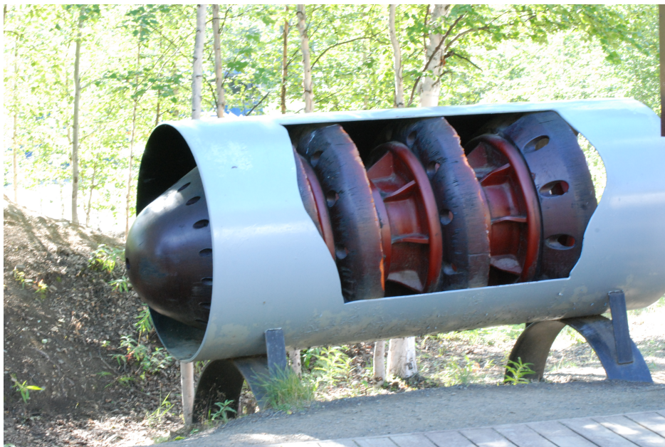
Cutaway Display of a PIG in a Pipe
