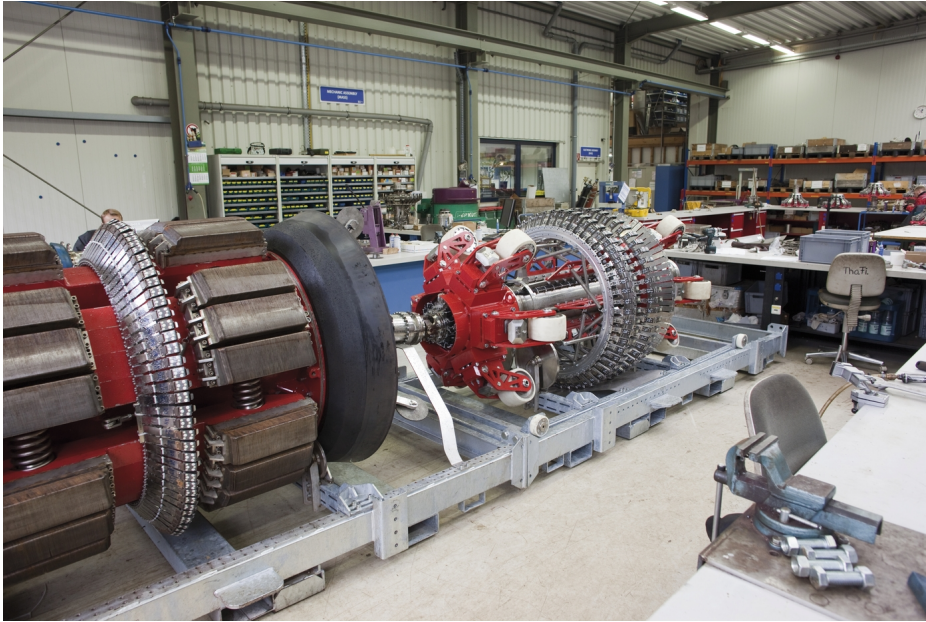
A Large, "Intelligent" PIG Used on Nordstream
