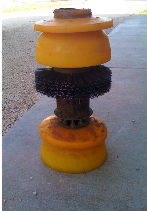
Simple PIG with Wire Brush for Cleaning
